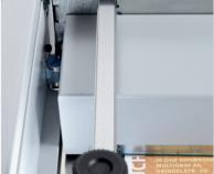
Two delivery sections The delivery side consists of two different output levels. For creasing and folding, the upper delivery belt is used, for creasing only the lower reception tray.
